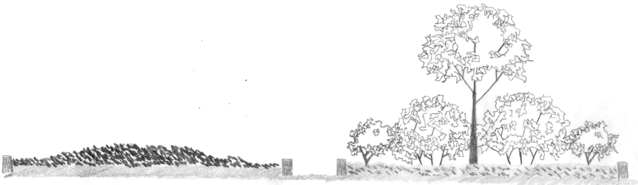
(Dig. 3) This is a section of how the Compost Commons would work. The bed on the right has been completed, the finished product being a planted bed. The bed on the left is still in progress, with a layer of soil on the bottom and the compostina materials on top.
